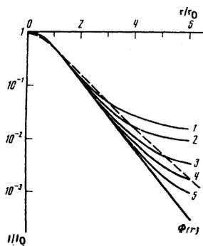
FIG. 3. Radial distribution of the intensity at various distances from the nonlinear focus (gaussian beam,  $P_0 = 5P_{cr}$ : 1)  $\Delta z = 4.5 \times 10^{-3} l_d$ ; 2)  $\Delta z = 1.1 \times 10^{-3} l_d$ ; 3)  $\Delta z = 1.5 \times 10^{-4} l_d$ ; 4)  $\Delta z = 1.3 \times 10^{-5} l_d$ ; 5)  $\Delta z = 2 \times 10^{-6} l_d$ .  $I_0$  is the intensity on the beam axis,  $r_0$  is the radius at the intensity level  $I = I_0/2$ , and the dashed line is the Townes intensity profile.
