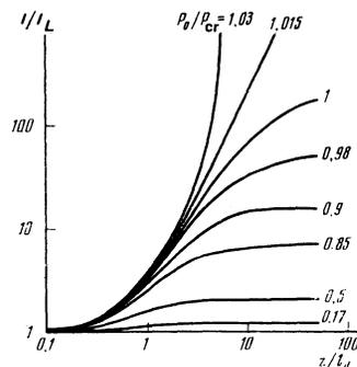
FIG. 4. Field intensity on the beam axis in a nonlinear medium at various  $P_0/P_{cr}$ .  $I_L$  is the field intensity in the absence of nonlinearity.
