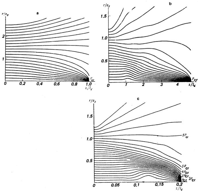
FIG. 1. Energy flux lines for beams with different intensity profiles: a) gaussian beam,  $N = 2$ ,  $P_0 = 1.5P_{cr}$ ; b) supergaussian beam  $N = 8$ ,  $P_0 = 1.5P_{cr}$ ; c)  $N = 8$ ,  $P_0 = 7P_{cr}$ ;  $a_0$  and  $l_d$  are the characteristic radius and diffraction length of the beam. The quantities marked on the figure correspond to the streamlines that limit the indicated power.
