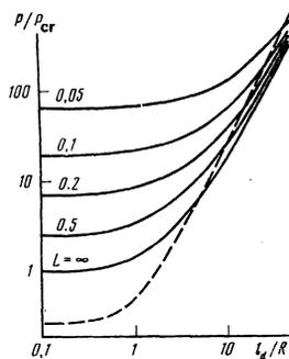
FIG. 5. Dependence of the self-focusing threshold on the divergence of the input beam for different medium nonlinearity lengths  $L$ . The dashed line is the plot obtained to the zero aberration approximation,  $R$  is the curvature radius of the phase front at the input, and  $l_d = ka_0^2$  is the diffraction length of the beam. The quantities marked on the figure correspond to the streamlines that limit the indicated power.
