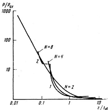
FIG. 2. Dependence of the self-focusing length on the input power for various values of  $N$ . The numbers indicate the annular zones for an  $N = 8$  supergaussian beam.
