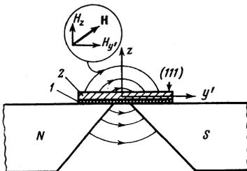
FIG. 1. Position of specimen and field distribution in the magnet that stabilizes the domain wall in a plane. 1)  $Y_{2.7}Bi_{0.3}Fe_{3.8}Ga_{1.2}O_{12}$  film; 2),  $Gd_3Ga_5O_{12}$  substrate.
