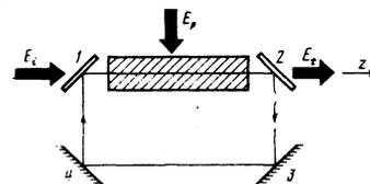
FIG. 2. Sample (shown shaded) placed in a ring resonator.
