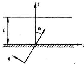
FIG. 1. Schematic representation of an experiment for observation of self-focusing in a plane cell with NLC. The polarization vector  $\mathbf{e}$  of the light wave lies in the  $xz$  plane; the wave is propagating in the cell with wave vector  $\mathbf{k}$ . In the plane  $z = 0$ , the orientation of the director is prescribed by rubbing or appropriate treatment of the wall of the cell. The transparent material of the wall is hatched. The free surface of the NLC is in the plane  $z = L$ .
