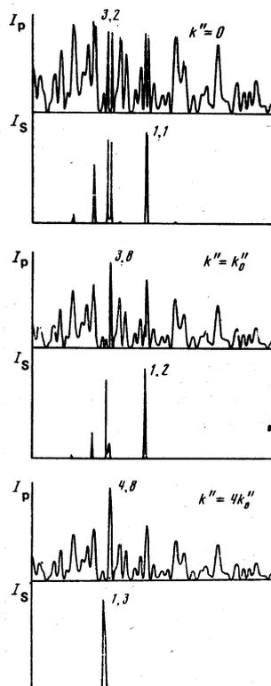
FIG. 8. Oscillograms of lasing at different values of the dispersion and at  $n = 25$ . The laser parameters and the realizations of the initial noise fields are the same as in Fig. 4.
