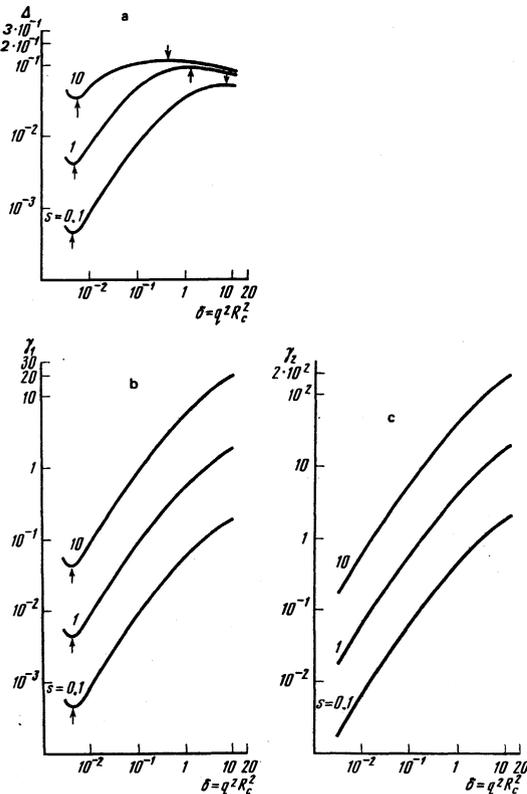
FIG. 1. Dependences of the depolarization coefficient  $\Delta$  (a) and of the quantities  $\gamma_1$  (b) and  $\gamma_2$  (c) on  $\delta = q^2 R_c^2$  for various values of the parameter  $s$ . The arrows identify the extrema.
