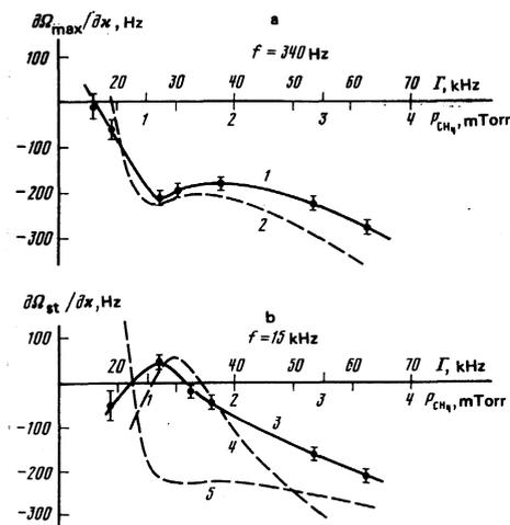
FIG. 2. Slope of the field shift of the resonance peak (a) and the stabilized frequency (b) versus methane pressure. Curves 1 and 3 represent the experimental results, and curves 2, 4, and 5 were calculated.
