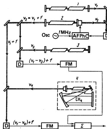
FIG. 1. Schematic diagram of the apparatus: 1, 3—stabilized lasers, 2—heterodyne laser, 4—laser with telescopic beam spreader, AFPhC—electronic automatic frequency and phase control system, Osc—rf oscillator, FM—frequency meter, D—photodetector.
