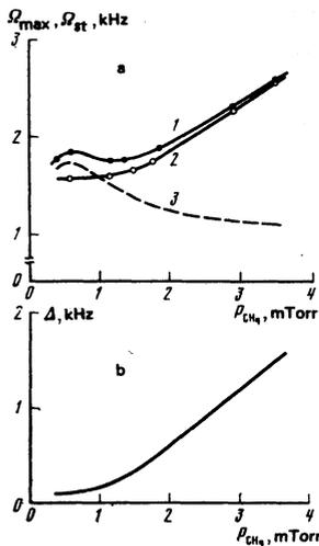
FIG. 3. a) Shift of the resonance peak (curve 1) and shift of the stabilized frequency (curve 2) of an He-Ne/ $CH_4$  laser versus methane pressure. Curve 3 shows the calculated shift of the resonance peak due to the effect of the MHFS. b) Collisional shift of the resonance peak in methane.
