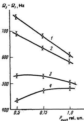
FIG. 4. Field shift of the stabilized frequency of the He-Ne/ $CH_4$  laser for various values of the magnetic field strength  $H$ : 1 -  $H = 0$ , 2 -  $H = 9$  Oe, 3 -  $H = 27$  Oe, 4 -  $H = 45$  Oe.
