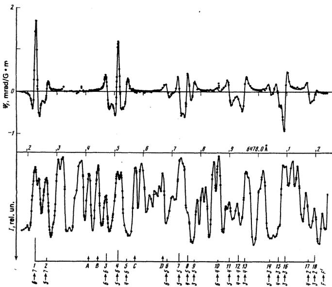
FIG. 6. Faraday rotation and absorption spectrum of bismuth vapor in the region of the  $\lambda = 648$  nm transition.
