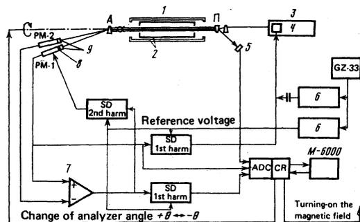
FIG. 3. Diagram of experiment: 1—oven and cell with Bi vapor, 2—magnetic screens, 3—laser, 4—selector, 5—photodiode, 6—attenuators, 7—subtraction circuit, 8—filter, 9—diffusers, SD—synchronous detector, GZ-33—sound generator, CR—control register.
