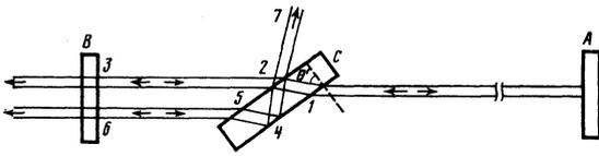
FIG. 4. Schematic representation of the position of the selector in the laser resonator: A, B—resonator mirrors, C—plane-parallel plate, 2—partly reflecting coating, 4—totally reflecting coating; for the remaining notation see the text.
