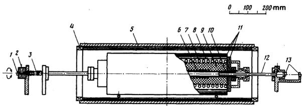
FIG. 5. Oven and cell with bismuth vapor: 1—analyzer prism, 2—entry of helium, 3—movable gasket, 4—coil, 5—steel housing, 6—heater, 7—cooling, 8—sectionalized coil, 9—thermal insulation, 10—ceramic cell, 11—magnetic screens, 12—collimators, 13—polarizer prism.
