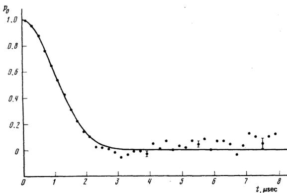
FIG. 9. Plot of  $P_0(t)$  in  $V_3Ga$ , obtained by summing 20  $N(t)$  distributions for the relaxation  $\mu^+$  signals at different values of  $H$  and  $T$ . The smooth curve is the Gaussian function  $P_0(t) = e^{-\sigma_0^2 t^2}$  at  $\sigma_0 = 0.711 \pm 0.007 \mu\text{sec}^{-1}$ .
