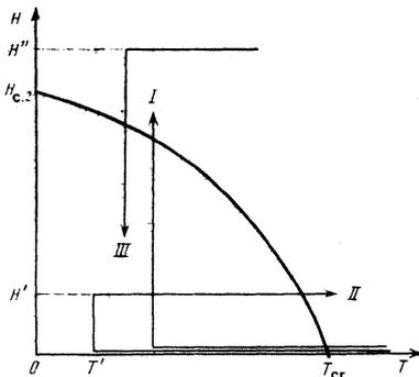
FIG. 2. Schematic representations of regimes I, II, and III of the variation of  $H$  and  $T$ , used in the present investigation of the superconductors  $V_3Ga$  and niobium. The continuous line separates the normal and superconducting states of the metal.
