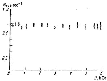
FIG. 7. Damping rate  $\sigma_0$  of the relaxation  $\mu^+$  signal in  $V_3Ga$  at  $T=11.5$  K for different values of the external magnetic field  $H$ .
