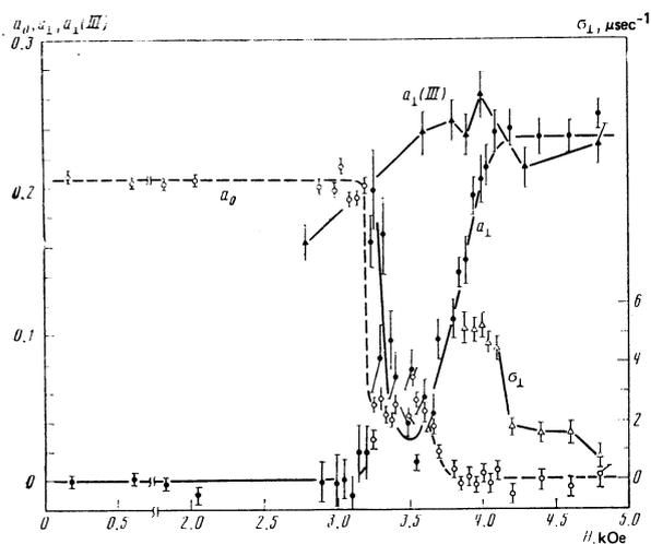
FIG. 5. The parameter  $a_0$  of the relaxation  $\mu^+$  signal and the parameters  $a_{\perp}$  and  $\sigma_{\perp}$  of the precession  $\mu^+$  signal in niobium vs. the field  $H$  at  $T = 4.3$  K, obtained in regime I;  $a_{\perp}$  (III) is the amplitude of the precession signal in regime III in a field  $H' = 4800$  Oe and at  $T = 4.3$  K (see Fig. 2). The continuous lines and the lines joining the experimental points are shown for clarity.
