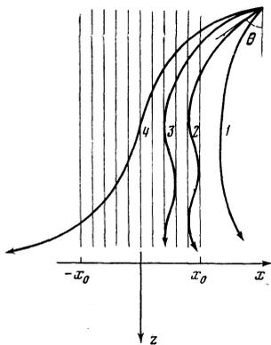
FIG. 4. Capture of particles into a magnetic channel: 1—reflection of slow particles; 2, 3—capture of particles with initial velocities  $|v_x|_2 < |v_x|_3 < |\Delta v_x^{\max}|$  into the elementary channel; 4—motion of uncaptured particle with  $|v_x|_4 > |v_x^{\max}|$ .
