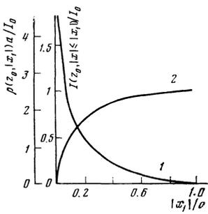
FIG. 2. Focusing characteristics at optimal channel length (curve 1 corresponds to the reduced particle-flux density  $\rho(z_0, x_1)$ ; curve 2 corresponds to the reduced integral flux  $I(z_0, |x| \leq |x_1|)$  in the region  $|x| \leq |x_1|$ ).
