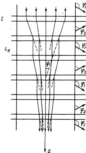
FIG. 3. Asymptotic focusing of particle flux by a multi-domain structure with alternating magnetization directions.
