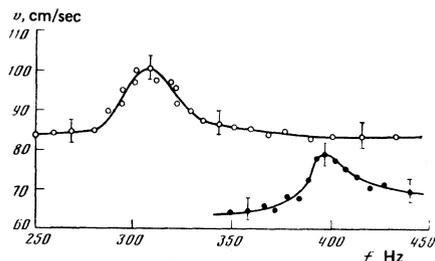
FIG. 2. Dependences of the self-pumping velocity on the pulse-repetition frequency (○—CO<sub>2</sub>, P=100 Torr, ●—air, P=200 Torr).
