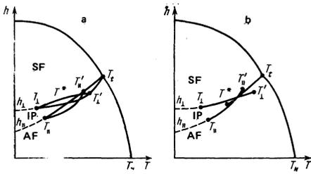
FIG. 3. Phase diagram of a uniaxial antiferromagnet ( $\beta < 0$ ). The dotted lines denote line of transition of the second kind to the IP from the AF and SF phases:  $T_{II}$ ,  $T_{I1}$ ,  $T_{II'}$ , and  $T_{I1'}$  are the terminal points of lines of phase transition of the first kind to the IP.
