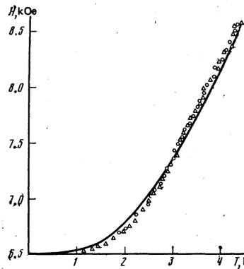
FIG. 4. Temperature dependence of the transition field  $h_{tr}$  for  $\text{CuCl}_2 \cdot 2\text{H}_2\text{O}$ . Points, results of experimental investigation by the AFMR method (according to the data of Ref. 7); triangles, results of experimental investigation by the NMR method. The solid line represents the results of a numerical calculation.
