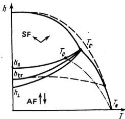
FIG. 2. Phase diagram of a uniaxial antiferromagnet ( $\beta > 0$ ). The dotted line shows the phase diagram of  $\text{GdAlO}_3$ ;<sup>5</sup> the dashed-dotted line represents the line  $h_{\sigma_1=0}(T)$ .
