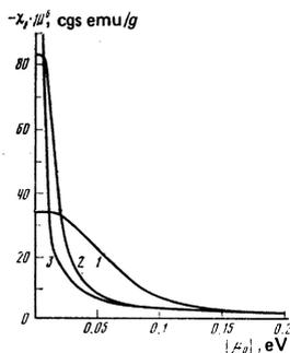
FIG. 4. Diamagnetic susceptibility of two-dimensional graphites as function of the position of the Fermi level ( $\gamma = 5 \cdot 10^{-4}$  eV) at the temperatures 300 (1), 77 (2), and 4.2 K (3).
