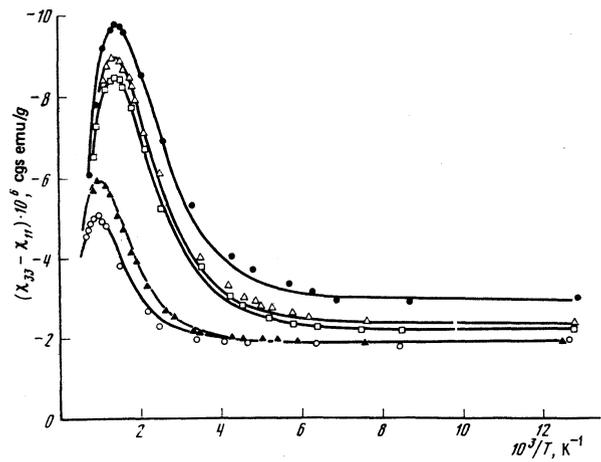
FIG. 3. Temperature dependence of the diamagnetic susceptibility of pyrocarbons with boron. The experimental data of Ref. 18 are represented by different symbols: ●—sample 40AS,  $\Delta$ —40AP,  $\square$ —56P,  $\blacktriangle$ —100P, and  $\circ$ —150S. Solid lines—calculated curves for the parameters  $A$  and  $\gamma$  listed in the table.
