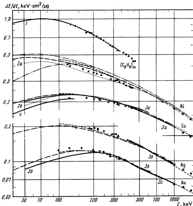
FIG. 1. Specific energy losses of hydrogen ions: 1 and □—Ref. 18, 2a and 2b—Ref. 15, 3a and 3b—Ref. 16, 4—Ref. 22, 5a, 5b, and 5c—Ref. 17, ■—Ref. 23, ●, ▲, ▼, ◆—present work (various targets). Curves with long and short dashes—results of the calculations of Refs. 30 and 29, respectively. Dash-dot curves with single and double dots—results of calculations of Ref. 32 without and with allowance for the change of the effective charge of the proton, respectively.
