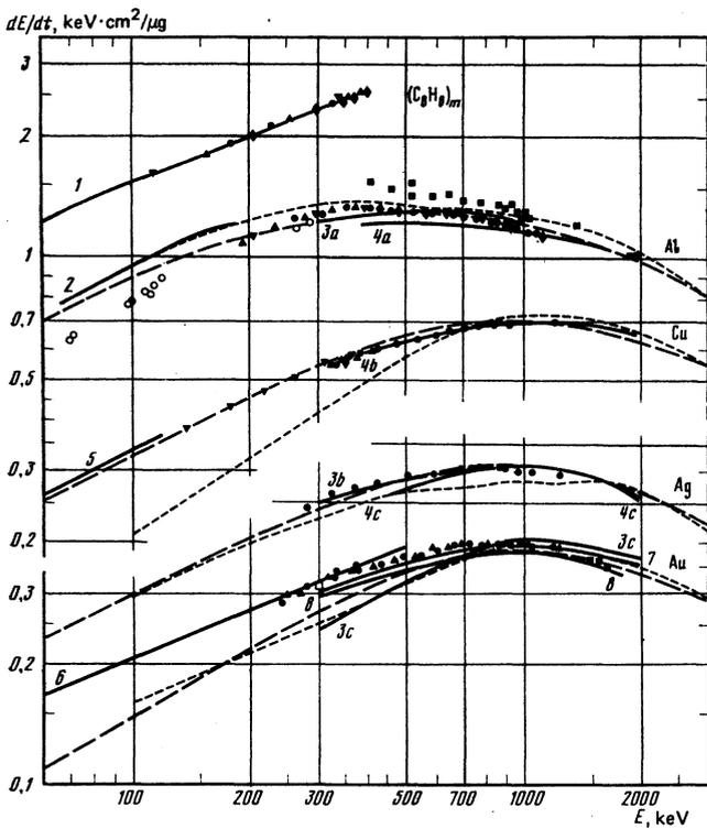
FIG. 2. Specific energy losses of helium ions: 1 and  $\square$ —Ref. 18, 2—Ref. 26, 3a, 3b, and 3c—Ref. 19, 4a, 4b, and 4c—Ref. 20, 5—Ref. 22, 6—Ref. 24, 7—Ref. 27,  $\circ$ —Ref. 25,  $\bullet$ ,  $\blacktriangle$ ,  $\blacktriangledown$ ,  $\blacklozenge$ —present work. Curves with long and short dashes—results of calculations of Refs. 31 and 29, respectively.
