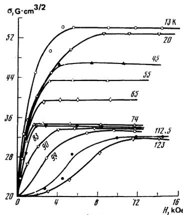
FIG. 3. Magnetization curves as functions of the field of the sample  $Cd_{0.487}In_{0.513}Cr_2Se_4$  at various temperatures.
