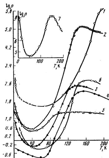
FIG. 1. Temperature dependence of  $\log \rho$  for the system of single crystals  $\text{Cd}_{1-x}\text{In}_x\text{Cr}_2\text{Se}_4$ : curve 1— $x = 0.047$ , 2—0.51, 3—0.513, 4—0.378, 5—0.58, 6—0.1; curve 7— $x = 0.012$ .
