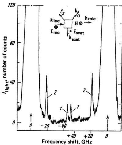
FIG. 7. Spectrum of scattering of light ( $\lambda = 632.8$  nm) at  $90^\circ$  in  $\text{CoCO}_3$  ( $T \lesssim 2$  K) by thermal  $y$  magnons (1) and by parametric  $y$  phonons (2), excited by microwave power with  $\nu_p = 36.2$  GHz under AFMR conditions.
