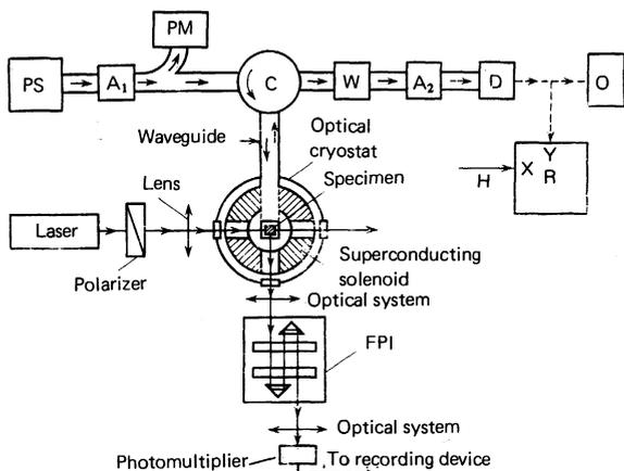
FIG. 1. Schematic drawing of the experimental setup for observation of light scattering when microwave power is fed to the specimen: FPI, Fabry-Perot interferometer; PS, microwave pumping source; A<sub>1</sub> and A<sub>2</sub>, attenuators; PM, microwave power meter; C, circulator; W, wavemeter; D, detector; O, oscilloscope; R, XY recorder.
