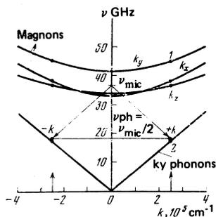
FIG. 8. Sketch illustrating parametric excitation of  $y$  phonons in  $\text{CoCO}_3$  under AFMR conditions at  $\nu_{\text{AFMR}} = 36$  GHz.
