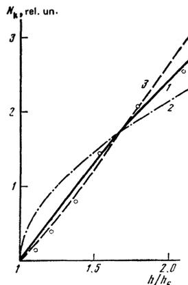
FIG. 6. Dependence of the number of parametric magnons  $N_k$  on the value of the excess of the microwave field above the threshold value,  $h/h_c$ . Curve 1 is plotted from formula (6), Curve 2 from formula (7), Curve 3 from formula (5). The experimental points correspond to Fig. 4.
