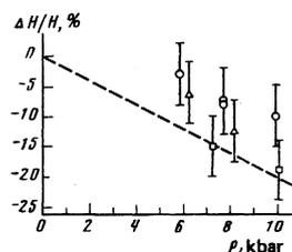
FIG. 2. Relative changes of the hyperfine magnetic fields at the  $^{57}\text{Fe}$  nuclei with changing pressure at  $T = 78$  K:  $\Delta$  – alloy with 0.5 at.% Fe,  $\circ$  – alloy with 1.5 at.% Fe,  $\square$  – alloy with 3.5 at.% Fe. Dashed line—pressure dependence of the magnetic moments of the Cr atoms for pure chromium (from the data of Ref. 9).
