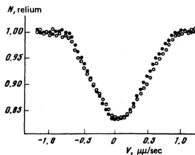
FIG. 1. Mössbauer spectra of  $^{57}\text{Fe}$  sample of an alloy of chromium with 1.5 at.% Fe at  $T = 78$  K:  $\circ$  – spectrum at atmospheric pressure,  $\bullet$  – at 9.9 kbar. The dimension of the point is equal to the statistical error. The Mössbauer source temperature is  $\sim 100$  K.
