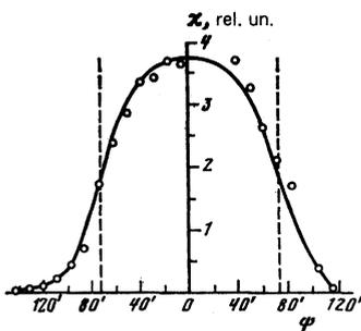
FIG. 4. Amplitude of the spike of the longitudinal component of the magnetic susceptibility in the orientational transition vs. the angle  $\psi$ .
