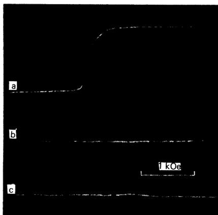
FIG. 1. Oscillograms of the longitudinal  $M_{\parallel}$  (a) and transverse  $M_{\perp}$  (b, c) components of the magnetization as functions of the magnetic field intensity in the region of the orientational transition ( $H_c = 175$  kOe). The magnetic field direction is close to that of the magnetic axis.
