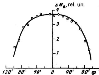
FIG. 6. Dependence of the jump of the longitudinal component of the magnetization in the orientational transition on the angle  $\psi$ .
