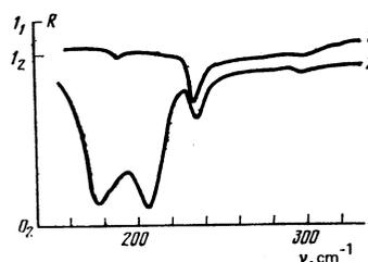
FIG. 2. IR reflection spectra of  $\text{CdS}_{1-x}\text{Se}_x$  ( $x \approx 0.1$ ) films in  $s$ -polarized light: 1 -  $d = 0.8 \mu\text{m}$ , 2 -  $d = 3.5 \mu\text{m}$ .
