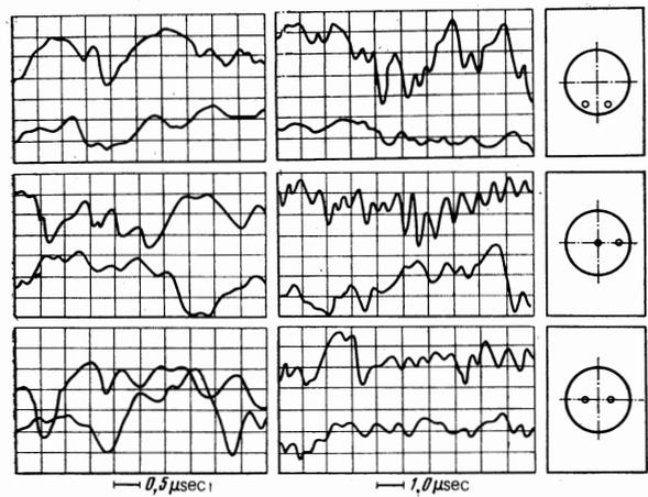
FIG. 4. Oscillograms of current density at two points of the cross section of the beam. On the right are shown arbitrarily the coordinates of the points.  $I_0 = 160$  mA,  $U_0 = 14$  kV, diameter 2.5 mm.
