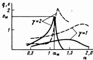
FIG. 2. Calculated dependences of the coefficients  $q$  (dashed) and  $s$  (solid curves) in formula (2) on the dimensionless frequency  $\alpha = \omega/\omega_i$ .
