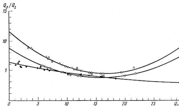
FIG. 2. Nonlinear signal registered by calorimeter  $PD_3$  and normalized to the total radiation energy, as a function of the total energy passing through the radiation system (arbitrary units):  $\square$ —LGS-27 sample in the first constriction,  $\triangle$ —the same sample in the fifth constriction, with different filters in front of the calorimeter  $PD_3$ ;  $\bullet$ —air.
