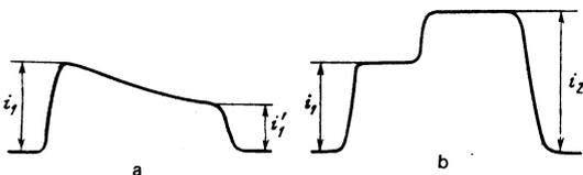
FIG. 2. Current pulse at  $\tau \ll T$  in single-phase (a) and two-phase (b) systems.
