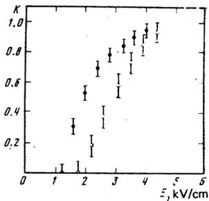
FIG. 4. Coefficient of electron emission from liquid (○) and solid (●) Xe vs. the electric field intensity inside the liquid (crystal).
