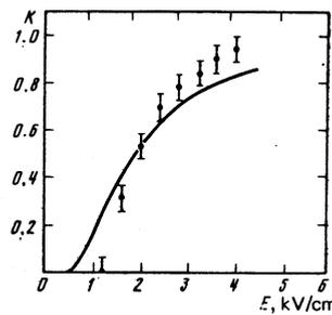
FIG. 5. Calculated (solid curve) and experimental (●) dependences of the coefficient of electron emission from solid Xe on the electric field intensity.
