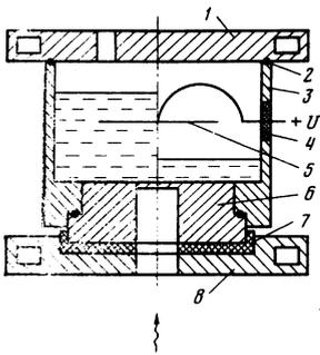
FIG. 1. Chamber for the measurement of the coefficient of electron emission from condensed noble gases. 1—Cover, 2—indium or teflon gasket, 3—housing, 4—high-voltage lead, 5—anode, 6—aluminum cathode liner, 7—insulating teflon insert, 8—bottom.
