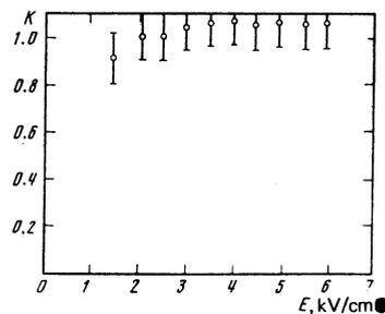
FIG. 3. Coefficient of electron emission from liquid Ar as a function of the electric field intensity inside the liquid.
