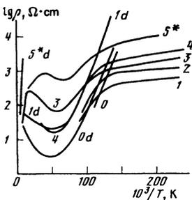
FIG. 3. Temperature dependences of the microwave resistivity of samples with chemical-donor concentrations  $N_d = 2 \cdot 10^{13} \text{ cm}^{-3}$  and different dislocation densities: curve 0—without dislocations; 1 —  $N_D = 2 \cdot 10^6 \text{ cm}^{-2}$ ; 2 —  $N_D = 6 \cdot 10^6 \text{ cm}^{-2}$ ; 3 —  $N_D = 9 \cdot 10^6 \text{ cm}^{-2}$ ; 4 —  $N_D = 1 \cdot 10^7 \text{ cm}^{-2}$ ; 5\* —  $N_D = 2 \cdot 10^7 \text{ cm}^{-2}$ .
