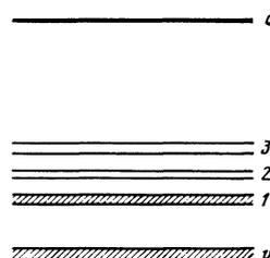
FIG. 4. Proposed energy level scheme of dislocations in germanium.
