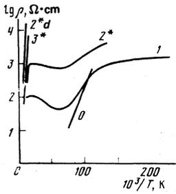
FIG. 2. Temperature dependences of microwave resistivity of samples with chemical-donor concentration  $N_d = 5 \times 10^{12} \text{ cm}^{-3}$  and with different dislocation densities: curve 0—without dislocations; 1 —  $N_D = 2 \cdot 10^6 \text{ cm}^{-2}$ ; 2\* —  $N_D = 6 \cdot 10^6 \text{ cm}^{-2}$ ; 3\* —  $N_D = 2 \cdot 10^7 \text{ cm}^{-2}$ .
