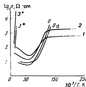
FIG. 1. Temperature dependences of the microwave resistivity of samples with chemical-donor concentration  $N_d = 3 \times 10^{12} \text{ cm}^{-3}$  and with various dislocation densities: curve 0—without dislocations; 1— $N_d = 3 \cdot 10^5 \text{ cm}^{-2}$ ; 2— $N_d = 2 \cdot 10^6 \text{ cm}^{-2}$ ; 3— $N_d = 5 \cdot 10^6 \text{ cm}^{-2}$ .
