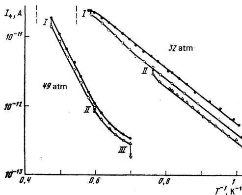
FIG. 7. Dependence of positive current on the temperature at a voltage 150 V before and after deformation at two pressures. The vertical dashed lines show the corresponding melting temperatures. The Roman numerals designate the sequence of the deformations.
