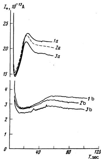
FIG. 3. Typical transient plots for positive current in the diode after application of a voltage 203 V—upper curves—or 73 V—lower curves—in a crystal with  $V_{\text{mol}} = 19.67 \text{ cm}^3$  at  $T = 1.67 \text{ K}$ . Curves 1 were obtained for an undeformed crystal, curve 2 for a crystal subjected to deformation at  $T_1 = 2.11 \text{ K}$ , and curves 3 after deformation at  $T_2 = 1.67 \text{ K}$ .
