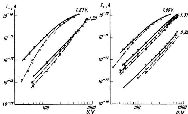
FIG. 5. Plots of positive and negative currents in a crystal with  $V_{\text{mol}} = 20.55 \text{ cm}^3$  before and after plastic deformation: ●—undeformed crystals; white circles—deformed crystal. In the left-hand diagram: ○— $T_1 = 1.67 \text{ K}$ , △— $T = 1.43 \text{ K}$ , ▽— $T_2 = 1.30 \text{ K}$ ; in the right-hand diagram:  $T_1 = 1.69 \text{ K}$ , △— $T_2 = 1.31 \text{ K}$ .
