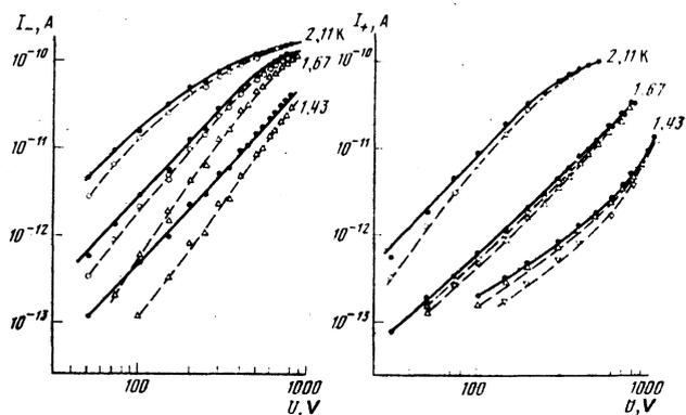
FIG. 6. Plots of positive and negative currents against the voltage in a crystal with  $V_{\text{mol}} = 19.67 \text{ cm}^3$  before and after plastic deformation: ●—undeformed crystal; ○— $T_1 = 2.11 \text{ K}$ , △— $T_2 = 1.67 \text{ K}$ , ▽— $T_3 = 1.43 \text{ K}$ .
