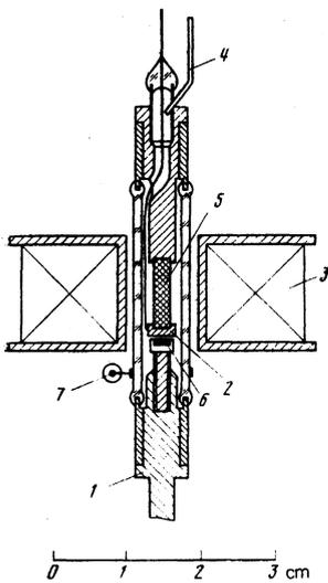
FIG. 1. Construction of the ampoule: 1—copper cold finger, 2—collector, 3—superconducting solenoid, 4—filling capillary, 5—magnetostrictor, 6— $\beta$ -active electrode, 7—resistance thermometer.
