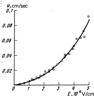
FIG. 9. Comparison of the function  $v(E)$  for negative charges in a crystal with  $V_{\text{mol}} = 20.23 \text{ cm}^3$  at  $T = 1.43 \text{ K}$  calculated from the current-voltage characteristics ( $\circ$ ) with the results of time-of-flight measurements in a triode ( $\bullet$ ).
