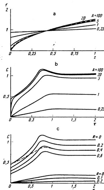
FIG. 10. Results of solution of the problem of the propagation of a chargefront in a diode: a) dependences of the relative electric field  $f$  on the coordinate  $z$  at the instant of time  $\tau=2$  in the absence of pinned charges; b) current transient curves in the absence of pinned charges; c) current transient curves with "strong" ( $A=100$ , upper curves) and "weak" ( $A=0.25$ , lower curves) source for a number of values of relative densities of the pinned charge  $R$ .
