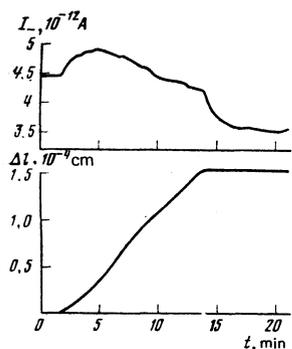
FIG. 2. Change of negative current in the course of plastic deformation in a crystal with  $V_{\text{mol}} = 20.55 \text{ cm}^3$  at a temperature 1.46 K.
