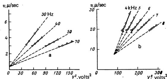
FIG. 2. Dependences of the velocity on the voltage across the cell: a) MBBA; b) PAA. The circles represent the velocities calculated from Eq. (1) and the triangles those calculated from Eq. (3).
