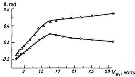
FIG. 5. Dependence of the angle of inclination of the molecules  $\Theta_0$  on the threshold voltage  $V_{th}$ . The circles represent the results calculated from Eq. (4) and the triangles those calculated from Eq. (5).
