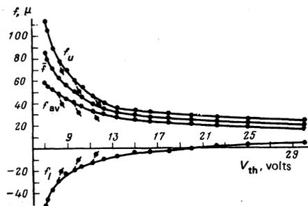
FIG. 4. Focal lengths for three positions of optical focusing by domains  $f_u$ ,  $f_{av}$ , and  $f_l$  plotted as a function of the threshold voltage  $V_{th}$  at  $t = 121^\circ\text{C}$ .
