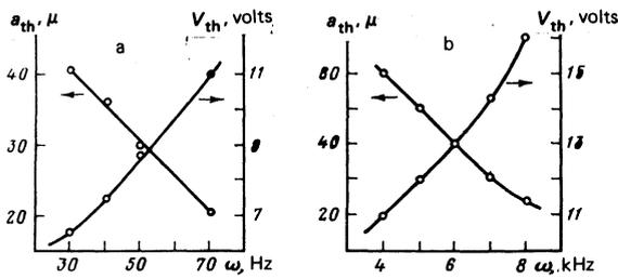
FIG. 3. Dependences of the threshold voltage  $V_{th}$  and diameter of a vortex tube  $a_{th}$  on the electric field frequency: a) MBBA; b) PAA.
