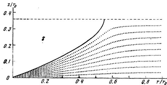
FIG. 7. Lines of constant electric potential calculated for  $\Delta/2r_{i0}=10^{-4}$  and  $a/2r_{i0}=0.4$ .
