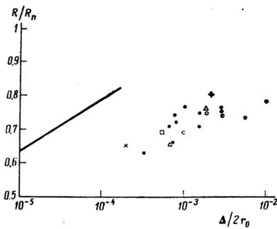
FIG. 9. Dependence of a resistance jump  $I=I_c$  on the surface tension. The continuous curve is calculated. The points represent various experimental data: +) Ref. 9; ●) Ref. 10; △) Ref. 11; □) Ref. 12; ×) Ref. 13; ○) Ref. 14.
