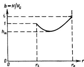
FIG. 8. Schematic distribution of the magnetic field in a normal metal outside the intermediate-state region.
