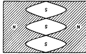
FIG. 4. General appearance of a periodic intermediate-state structure (the normal regions are shown shaded) in the case  $I = I_c$ ,  $\Delta/2r_{i0} = 3 \times 10^{-5}$  and  $a/2r_{i0} = 0.3$ .
