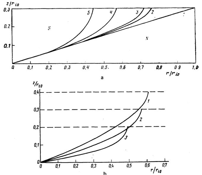
FIG. 5. Equilibrium phase interfaces. a) Results obtained for  $a/2r_{i0} = 0.3$  and different values of the surface tension: 1) original London structure ( $\Delta = 0$ ); 2)  $\Delta/2r_{i0} = 1.7 \times 10^{-5}$ ; 3)  $\Delta/2r_{i0} = 3 \times 10^{-5}$ ; 4)  $\Delta/2r_{i0} = 10^{-4}$ ; 5)  $\Delta/2r_{i0} = 3 \times 10^{-4}$ . b) Results for  $\Delta/2r_{i0} = 10^{-4}$  and different values of the structure period: 1)  $a/2r_{i0} = 0.4$ , 2)  $a/2r_{i0} = 0.3$ ; 3)  $a/2r_{i0} = 0.2$ .
