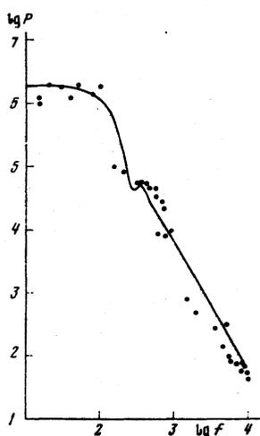
FIG. 11. Dependence of the logarithm of the power (in relative units) on the logarithm of the frequency in hertz. The continuous curve is calculated using Eq. (10) and the points are the results taken from Ref. 14.
