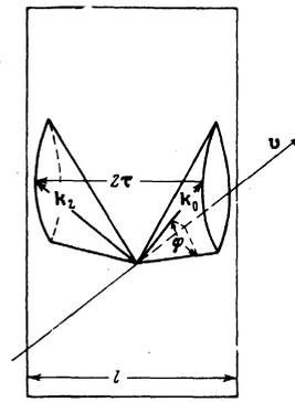
FIG. 1. Angular distribution of Vavilov-Cerenkov radiation in a cholesteric liquid crystal ( $k_0$  and  $k_2$  are wave vectors corresponding to radiation on the Cerenkov and diffraction cones, respectively, and  $\tau$  defines the orientation of the optic axis of the CLC).
