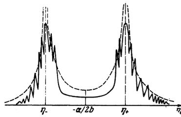
FIG. 3. Angular dependence of the amplitude of the wave emitted into the diffraction cone in an infinite CLC (broken curve) and in a finite specimen (solid curve).
