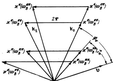
FIG. 2. Fine structure (polarization splitting) of Cerenkov and diffraction cones.
