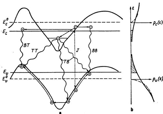
FIG. 1. Energy band diagram (a) and density of states distribution (b) in a disordered semiconductor. The shaded regions represent localized carrier states ( $E_c$  and  $E_v$  are the electron and hole percolation levels,  $E_c^0$  and  $E_v^0$  are the edges of the forbidden band of the undoped semiconductor). The wavy lines represent possible types of radiative transition.
