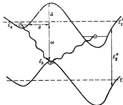
FIG. 2. Schematic representation of the emission of a photon in the case of an energy deficit  $\Delta$ .
