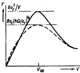
FIG. 3. Nonlinear dependence of damping force on the dislocation velocity. The notation is the same as in Fig. 2.
