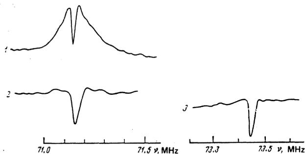
FIG. 1. First derivative of NMR signal for hematite crystals: 1—slowly cooled crystals, 295 K, 2—quenched crystals, 295 K, 3—crystals following any heat treatment, 77 K.
