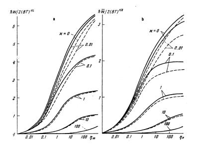
shows the band width  $\overline{W}$  averaged over the angles of emission of the photon from the gas layer.
