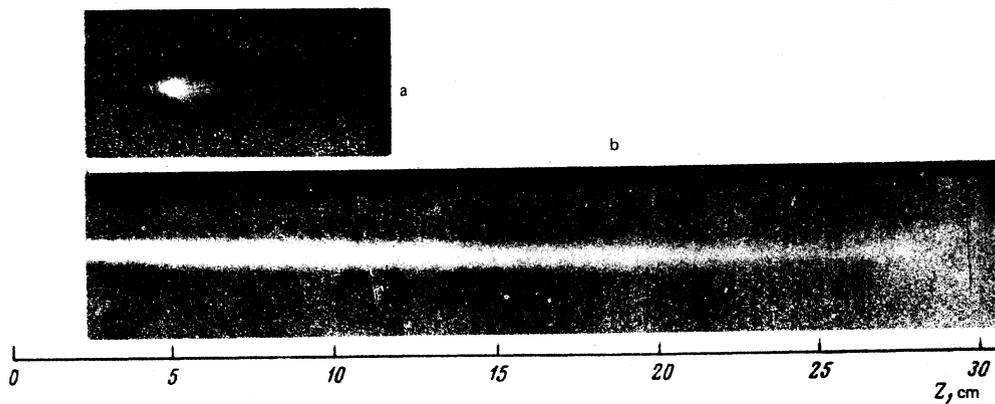
FIG. 2. Photographs of the beam with small (a) and deep (b) modulation of current density. The parameters of the beam-plasma system are as follows:  $I_{b0} = 3$  mA,  $U_0 = 300$  eV,  $P = 5.8 \times 10^{-3}$  Torr. Modulation frequency  $f = \Omega/2\pi = 400$  MHz, a)  $I_b/I_{b0} = 3 \times 10^{-2}$ , b)  $I_b/I_{b0} \sim 1$ .
