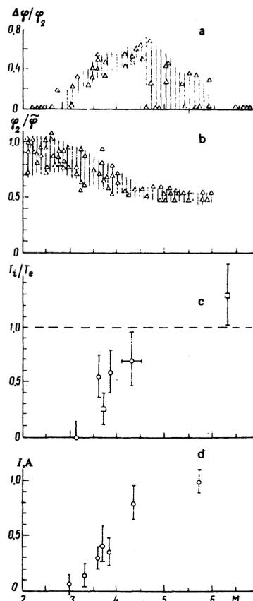
FIG. 2. Dependence of the following shock-wave parameters on the Mach number: a—of the relative amplitude of the isomagnetic potential discontinuity; b—of the ratio of the amplitude of the potential barrier to the decrease of the ion kinetic energy in the shock wave; c—of the ratio of the ion and electron temperatures behind the front; d—of the ion current (in amperes), which is proportional to the number of ions reflected from the potential barrier.
