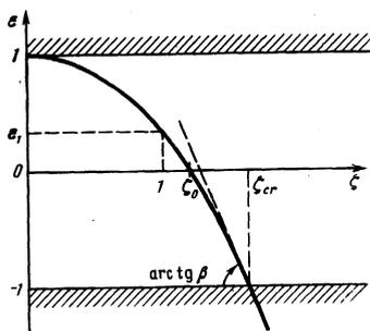
FIG. 4. Approximate variation of the energy of the level  $\epsilon$  with increasing  $\zeta = Z\alpha$ .
