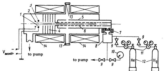
FIG. 1. Experimental setup: 1—electron beam, 2—annular cathode, 3—accelerating electrode, 4—gas delay line, 5—outer tube, 6—inner tube that limits the working volume, 7—electromagnetic valve, 8—volume ahead of valve, 9—valve, 10—manometer, 11—pressure reducer, 12—gas flasks, 13—windows for spectroscopic diagnostics, 14—magnetic-field coils.
