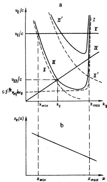
FIG. 1. Instability threshold of the plasma (a). The region of localization of the instability (b). The relatively small change in the amplitude of the pump wave inside the region of localization of the instability is neglected.
