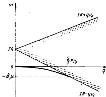
FIG. 1. Spin-wave dispersion law for a ferromagnetic exchange interaction  $I > 0$ .
