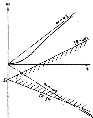
FIG. 2. Spin-wave dispersion law for an antiferromagnetic exchange interaction  $I < 0$ .
