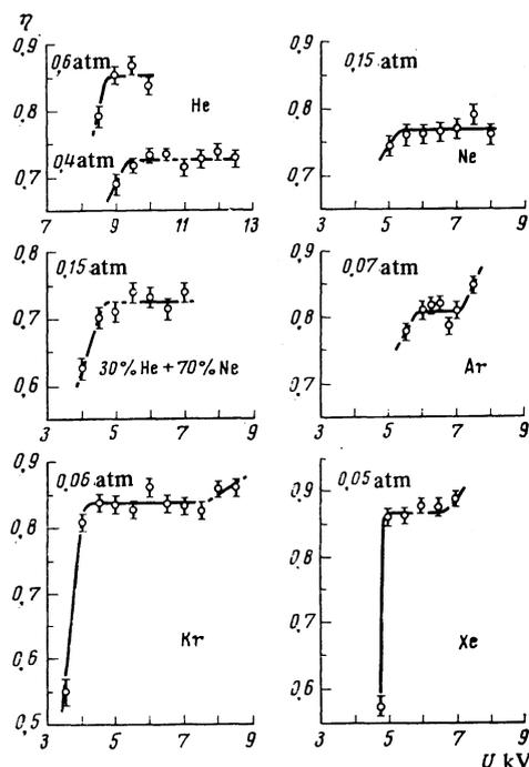
FIG. 2. Dependence of the efficiency  $\eta$  of a low-pressure spark chamber filled with a noble gas on the amplitude  $U$  of the high-voltage pulse ( $RC = 0.2 \mu\text{sec}$ ,  $t_d = 0.2 \mu\text{sec}$ ,  $t = 20^\circ\text{C}$ ).
