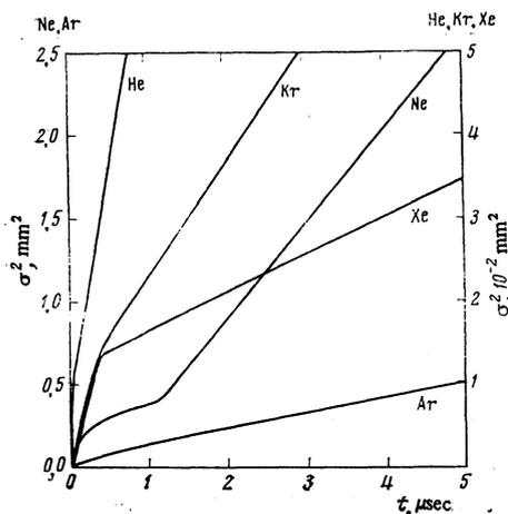
FIG. 4. Dependence of the mean square departure<sup>[21]</sup> of the electron on the delay time  $t$  in noble gases under normal conditions.
