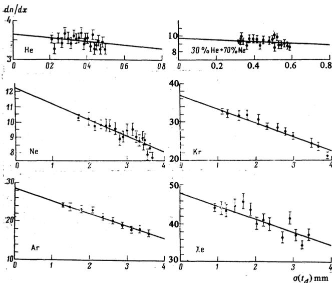
FIG. 3. Dependence of the specific primary ionization  $dn/dx$ ,  $\text{cm}^{-1}$ , on the calculated diffusion mean square displacement  $\sigma(t_d)$  of the electrons, formed by the charged particle in the gas (the results of one of cycles of measurements referred to normal conditions, are shown).
