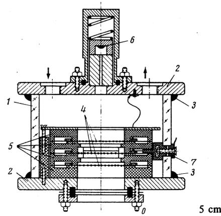
FIG. 1. Construction of the low pressure spark chamber: 1—glass case, 2—chamber cover, 3—vacuum cement, 4—wire electrodes, 5—teflon rings, 6—radioactive source ( $\text{Sr}_{88}^{90}$ ), 7—high-voltage lead.
