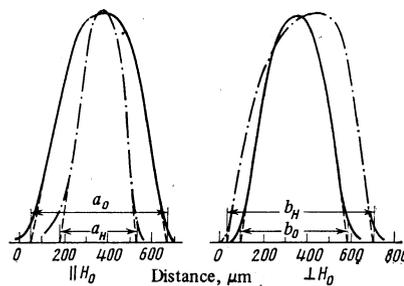
FIG. 5. Spatial distribution of the radiation of a large EHD in sample 5 at 1.8 K for  $H_0 = 0$  and  $H_0 = 10$  kOe, obtained by scanning in directions parallel and perpendicular to  $H_0$ ;  $F \parallel [111]$ ,  $H_0 \parallel [211]$ .
