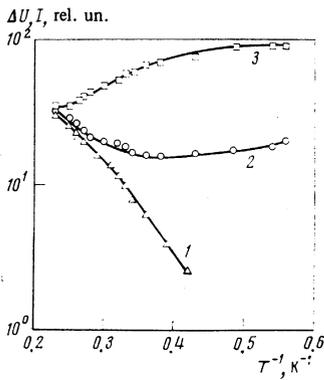
FIG. 4. Temperature dependence of RF absorption  $\Delta U$  in samples 3 (1) and 4 (2) and of the intensity  $I$  of the recombination radiation (3) in the absence of deformation at an excitation power 100 mW.
