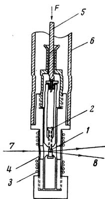
FIG. 1. Setup for the investigation of RF absorption and for the production of inhomogeneous deformation in germanium: 1—sample, 2—caprone screw, 3—high-frequency coil, 4—brass screen, 5—rod to transmit the deforming force and internal conductor of coaxial lead-in, 6, 7—exciting radiation, 8—recombination radiation.
