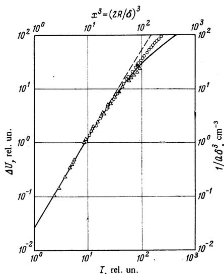
FIG. 2. Dependence of the RF absorption  $\Delta U$  on the recombination-radiation intensity  $I$  at  $F \parallel [111]$  and 1.8 K:  $\circ$ —for sample 5,  $\triangle$ —for sample 3;  $\bullet$ ,  $\blacktriangle$ —points at which the absolute values of  $R$  and  $\Delta U/U$  were measured. The dependence of  $1/Q\delta^3$  on  $x^3$  (solid line) was calculated in accordance with (2), (3), and (5).
