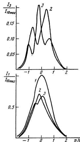
FIG. 3. Evolution of the pumping and third-harmonic pulses at  $\theta_0 = 2.2\pi$  and  $|\beta| = 2$ : 1—pumping pulse at the entrance; 2, 3—pulses at  $z = l_n$  and  $z = 2l_n$ .
