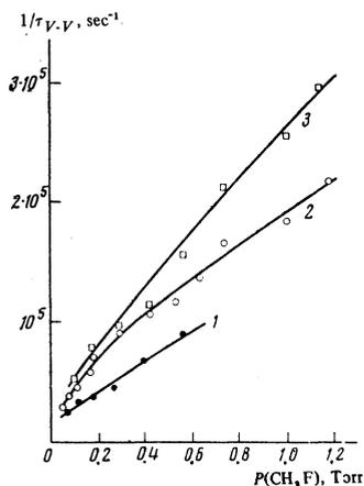
FIG. 4. Dependence of the time for energy transfer to  $\text{CH}_4$  molecules as a function of  $\text{CH}_3\text{F}$  pressure for  $P(\text{CH}_4) = 0.174$  Torr,  $\bullet - P(\text{Ar}) = 6$  Torr,  $\circ - P(\text{Ar}) = 20$  Torr,  $\square - P(\text{Ar}) = 70$  Torr.
