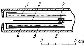
FIG. 2. Diagram of the source apparatus: 1—source crucible (tube with wall thickness  $\sim 0.5$  mm), 2—ceramic insulator, 3—needle 1 mm in diameter, 4—heater, 5—heat shields, 6—enclosure. Parts 1 and 3 are made of stainless steel and are joined by an insulating vacuum seal 2.
