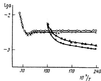
FIG. 3. Temperature dependence of the microwave conductance for deformed samples with dislocation density  $3 \times 10^5 \text{ cm}^{-2}$  ( $\bullet$ ),  $5 \times 10^5 \text{ cm}^{-2}$  ( $\blacktriangle$ ),  $1 \times 10^7 \text{ cm}^{-2}$  ( $\circ$ ), and  $5 \times 10^6 \text{ cm}^{-2}$  ( $\times$ ) at  $N_A = 2 \times 10^{12} \text{ cm}^{-3}$ .
