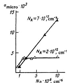
FIG. 4. Dependence of the microwave conductance on the dislocation density at  $T = 4.2 \text{ K}$  for deformed samples with initial acceptor concentration  $2 \times 10^{12} \text{ cm}^{-3}$  ( $\Delta$ ) and  $7 \times 10^{13} \text{ cm}^{-3}$  ( $\blacktriangle$ ).
