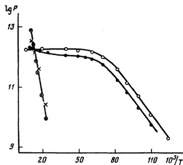
FIG. 2. Temperature dependence of the free-hole density in a control sample ( $\circ$ ) and deformed samples with dislocation density  $5 \times 10^5 \text{ cm}^{-2}$  ( $\bullet$ ),  $5 \times 10^6 \text{ cm}^{-2}$  ( $\times$ ), and  $1 \times 10^7 \text{ cm}^{-2}$  ( $\odot$ ) at  $N_A = 2 \times 10^{12} \text{ cm}^{-3}$ .
