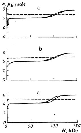
FIG. 2. Magnetization,  $\sigma$ , of a single-crystal iron garnet  $\text{Er}_{0.12}\text{Y}_{2.88}\text{Fe}_5\text{O}_{12}$  at 4.2 K as a function of the field: a) H along [111], b) H along [110] c) H along [100] (solid lines); dashed line—magnetization of yttrium iron garnet.
