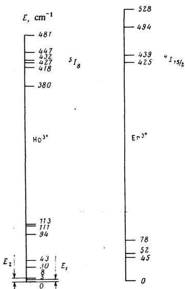
FIG. 1. Energy splitting of the ground multiplet of  $\text{Ho}^{3+}$  and  $\text{Er}^{3+}$  in yttrium iron garnet.
