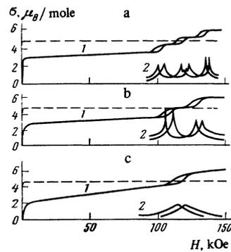
FIG. 3. Magnetization (1) and differential susceptibility (2) of a single crystal iron garnet  $\text{Ho}_{0.25}\text{Y}_{2.75}\text{Fe}_5\text{O}_{12}$  at 4.2 K as a function of the field: a) H along [111], b) H along [110], c) H along [100] (solid lines); dashed lines—magnetization of yttrium iron garnet.
