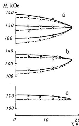
FIG. 4. Temperature dependence of the fields at which magnetization jumps occur in  $\text{Ho}_{0.25}\text{Y}_{2.75}\text{Fe}_5\text{O}_{12}$  (solid lines—field increasing, dashed lines—field decreasing); a) H along [111], b) H along [110], c) H along [100].
