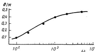
FIG. 5. Frequency dependence of the phase delay of the light flux. Points—experiment, curve—calculation by formula (15) with  $\tau=4 \times 10^{-3}$  sec.
