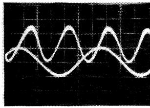
FIG. 4. Oscilloscope of oscillations of external field (lower trace) and of the photomultiplier current (upper trace) in a phase-frequency experiment; sweep rate 0.5 msec/cm of screen,  $\omega=2 \times 10^3 \text{ rad}^{-1}$ .
