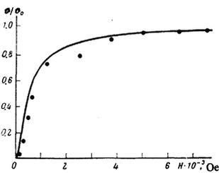
FIG. 2. Dependence of the phase difference between the ordinary and extraordinary rays on the intensity of the constant external field,  $T=297$  K. Points—experiment, curve—calculation by formula (10).
