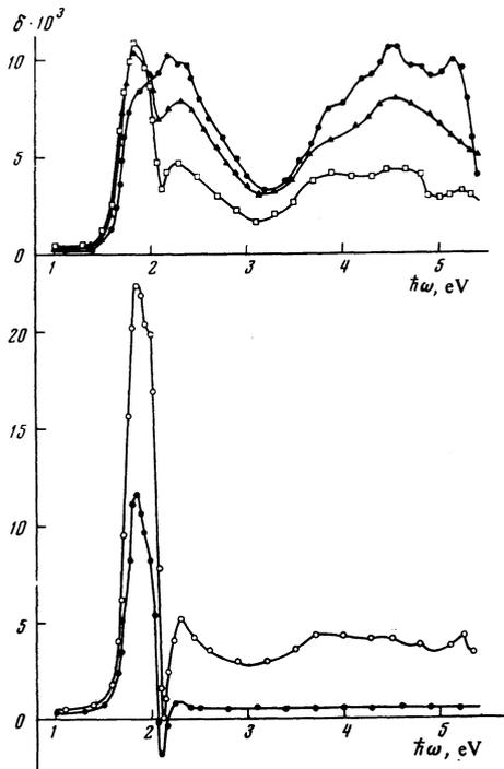
FIG. 6. Equatorial Kerr effect for the system of polycrystalline spinels  $\text{CoCr}_x\text{Fe}_{2-x}\text{O}_4$  ( $x = 0, 0.25, 0.5, 0.75, 1.0$ ),  $\varphi = 60^\circ$ : ●— $x = 0$ ; ▲— $x = 0.25$ ; □— $x = 0.5$  (top figure). ○— $x = 0.75$ ; ●— $x = 1.0$  (bottom figure).
