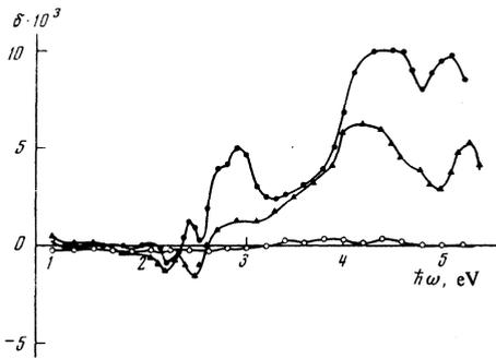
FIG. 8. Equatorial Kerr effect for the system of polycrystalline spinels  $\text{NiCr}_x\text{Fe}_{2-x}\text{O}_4$  ( $x=0, 0.5, 1.0$ ),  $\varphi=60^\circ$ ;  $\bullet$ — $x=0$ ;  $\blacktriangle$ — $x=0.5$ ;  $\circ$ — $x=1.0$ .
