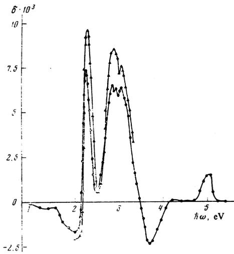
FIG. 2. Equatorial Kerr effects for single-crystal hematite  $\alpha\text{-Fe}_2\text{O}_3$  in the planes (111) and (100) at  $\varphi = 70^\circ$ :  $\bullet$ —(111) plane  $\blacktriangle$ —(100) plane.
