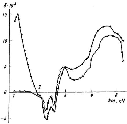
FIG. 5. Equatorial Kerr effect for single-crystal spinels  $\text{Ni}_{0.69}^{2+}\text{Fe}_{0.31}^{2+}\text{Fe}_2\text{O}_4$  and the film  $\text{NiFe}_2\text{O}_4$  ( $\varphi = 65^\circ$ ): ●—single crystal  $\text{Ni}_{0.69}^{2+}\text{Fe}_{0.31}^{2+}\text{Fe}_2\text{O}_4$ , (110) plane; ○— $\text{NiFe}_2\text{O}_4$  film, (100) plane.
