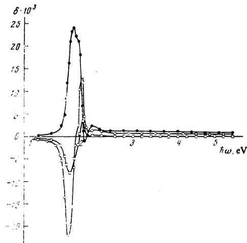
FIG. 7. Equatorial Kerr effect for single-crystal spinel  $\text{CoCrFeO}_4$  at different light-incidence angles: ●— $\varphi = 65^\circ$ , ○— $\varphi = 70^\circ$ , □— $\varphi = 75^\circ$ .
