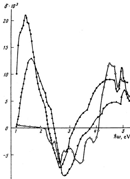
FIG. 4. Equatorial Kerr effect for magnetite  $\text{Fe}_3\text{O}_4$ :  $\bullet$ —bulky single-crystal sample of  $\text{Fe}_3\text{O}_4$  at  $\varphi = 65^\circ$ , (110) plane;  $\blacktriangle$ —the same at  $\varphi = 70^\circ$ ;  $\circ$ —single-crystal film of  $\text{Fe}_3\text{O}_4$  at  $\varphi = 65^\circ$  ((100) plane).
