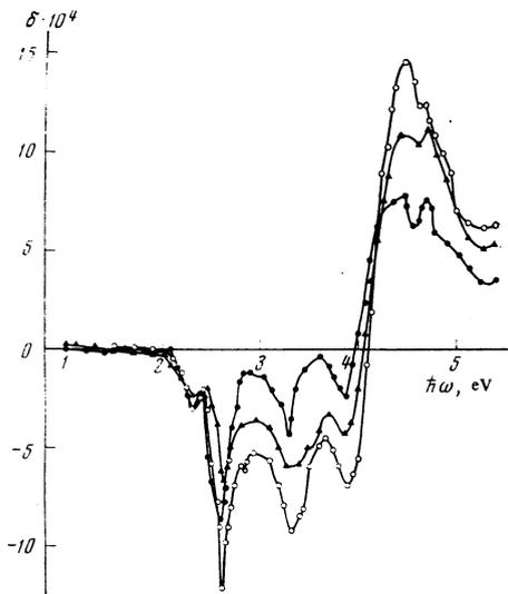
FIG. 3. Equatorial Kerr effect for the spinels  $\text{MgFe}_2\text{O}_4$  and  $\text{Li}_{0.5}\text{Fe}_{2.5}\text{O}_4$  at  $\varphi = 65^\circ$ :  $\bullet$ —single crystal  $\text{Li}_{0.5}\text{Fe}_{2.5}\text{O}_4$  ((110) plane),  $\blacktriangle$ —polycrystal  $\text{MgFe}_2\text{O}_4$ ,  $\circ$ —single-crystal film  $\text{MgFe}_2\text{O}_4$  ((100) plane).
