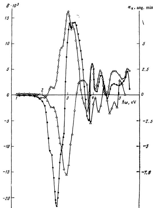
FIG. 1. Equatorial and polar Kerr effects for the single-crystal orthoferrite  $YFeO_3$  ((100) plane): ○—light incidence angle  $\varphi = 65^\circ$ , ●—light incidence angle  $\varphi = 70^\circ$ , Δ—polar Kerr effect ( $\varphi = 0^\circ$ ).
