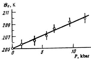
FIG. 2. The variation of the Curie temperature of a Pd-Co alloy (4.7 at. %) under hydrostatic pressure.
