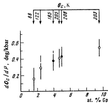
FIG. 3. Dependence of the quantity  $d\Theta_c/dP$  on the cobalt content in palladium. The points ● are data for Pd-Co alloys with a tin impurity (0.12 at. %).
