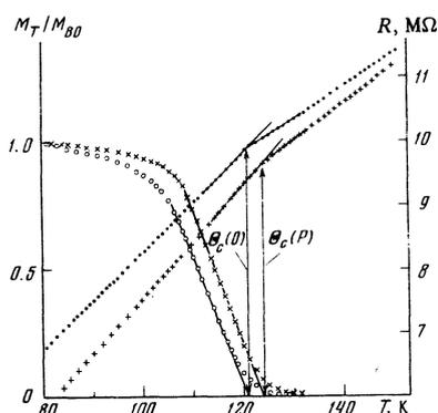
FIG. 1. Temperature dependence of the resistance, ( $\bullet$ ,  $+$ ), and of the magnetic moment, ( $\circ$ ,  $\times$ ), for a Pd-Co alloy (2.4 at.%) (simultaneous measurements):  $\circ$ ,  $\bullet$ ) without hydrostatic pressure;  $\times$ ,  $+$ ) under a pressure  $\sim 8.0$  kbar. The magnitude of the moment of the sample at any temperature has been expressed relative to the moment at 80 K.
