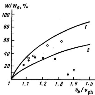
FIG. 5. The energy losses of the beam as a function of the beam velocity: 1) computed from the formula (7); 2) computed from the formula (8). The measured maximum values of the energy stored in the wave: (●) initial amplitude of the wave was 17.5 V; (○) 25 V.
