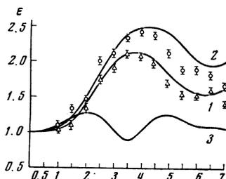
FIG. 3. Dependence of the wave amplitude on distance—comparison of the computer calculation with experiment. The initial wave amplitude is fixed;  $v_{ph} = 1.8 \times 10^7$  m/sec. The curve 1) is for  $v_b = 1.15v_{ph}$ ; 2) for  $v_b = 1.3v_{ph}$ ; 3) for  $v_b = 1.5v_{ph}$ . The experimental points:  $\circ$ ) are for  $v_b = 2.4 \times 10^7$  m/sec;  $\Delta$ ) for  $v_b = 2 \times 10^7$  m/sec.
