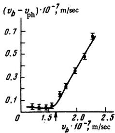
FIG. 2. Dependence of  $(v_b - v_{ph})$  on  $v_b$ . At the point marked by the arrow  $v_b = v_c$ .
