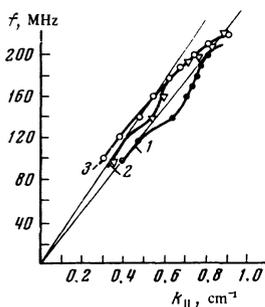
FIG. 1. Dispersion dependences: 1) plasma waveguide with a beam with  $v_b = 1.6 \times 10^7$  m/sec; 2) plasma waveguide with a beam with  $v_b = 1.9 \times 10^7$  m/sec; 3) plasma waveguide without a beam.
