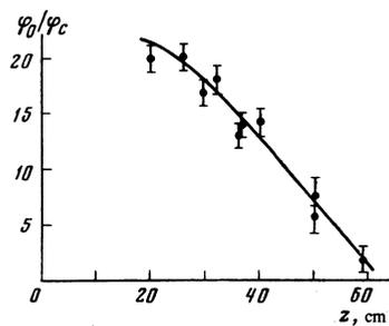
FIG. 4. Dependence of the distance over which the maximum of the wave amplitude is attained on the initial signal amplitude.
