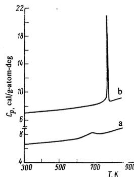
FIG. 1. Dependence of the specific heat of Pr (curve a) or Nd (curve b) on the temperature.
