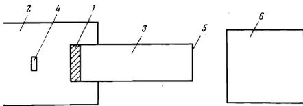
FIG. 1. Experimental setup: 1—sample (diameter 50 mm, thickness 50–25 mm); 2—large chamber; 3—small chamber; 4—striker (diameter 50 mm, thickness 5 mm); 5—transparent glass; 6—FÉU-38 radiation detector, oscilloscope, and photographic camera or UMI-93 image converter and photographic camera or ISP-51, image converter and photographic camera or UM-2 monochromator, photomultiplier, oscilloscope, and photographic camera.
