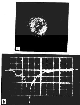
FIG. 5. Radiation of copper sample in the case of strong deformation without visible breaks,  $h = 27$  mm,  $p \approx 10^{-5}$  Torr: a) photograph obtained with an image converter, b) corresponding oscillogram,  $t_{\text{sweep}} = 0.5$  msec/div,  $U = 50$  mV/div.
