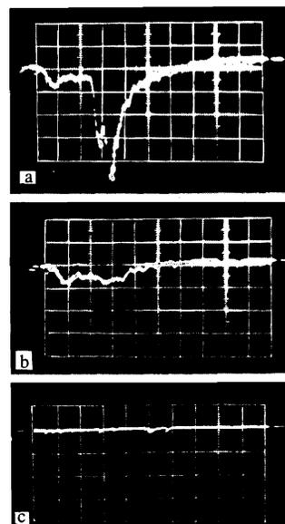
FIG. 3. Photomultiplier-signal oscillograms obtained upon destruction of a metal sample,  $t_{\text{weep}} = 0.5$  msec/div  $p \approx 10^{-5}$  Torr: a) breaking of rear surface, sample thickness  $h = 27$  mm, sensitivity of detecting system  $U = 50$  mV/div; b) deformation without visible break,  $h = 27$  mm,  $U = 50$  mV/div; c) undeformed rear surface,  $h = 50$  mm,  $U = 10$  mV/div.
