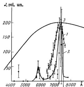
FIG. 6. Spectrum of emission produced when a copper sample is destroyed: 1—results of the reduction of the data obtained with the aid of a spectrograph and an electron-optical converter; 2—results of the reduction of the data obtained with the aid of a monochromator and a photomultiplier; 3—radiation of absolute black body heated to 4000°K. The error fields were determined from the results of the reduction of six spectra. The probable errors of  $\rho = 2\sigma/3$  are indicated.
